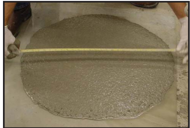
Figure 1 SCC with a slump flow of 29" (735 mm) as tested by the slump flow test
