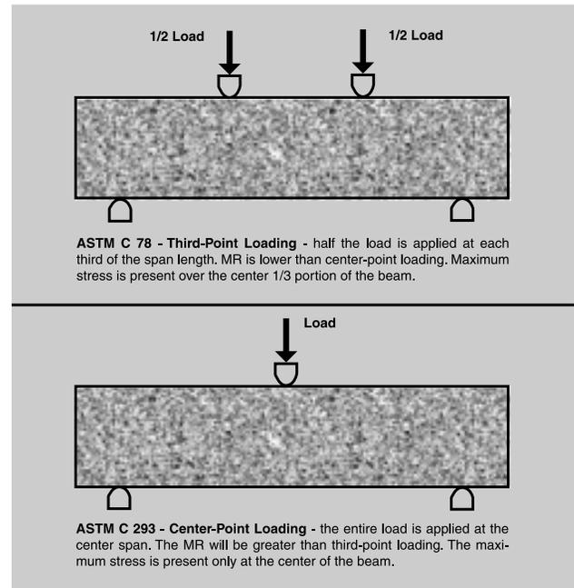
ets. For higher slump, after rodding, tap the molds to release air pockets and spade along the sides to consolidate. *Never allow the beam surfaces to dry at any time.* Immerse in saturated limewater for at least 20 hours before testing.
